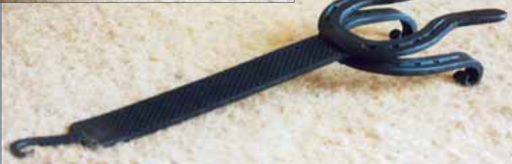
Made with non slip tempered rasp and forged horse shoes
